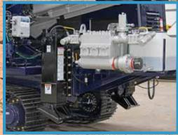
Optional on-board Aplex mud pump, which delivers up to 312 g/min. The build-in mud pump reduces transportation problems and increases maneuverability of the horizontal drilling machine.
