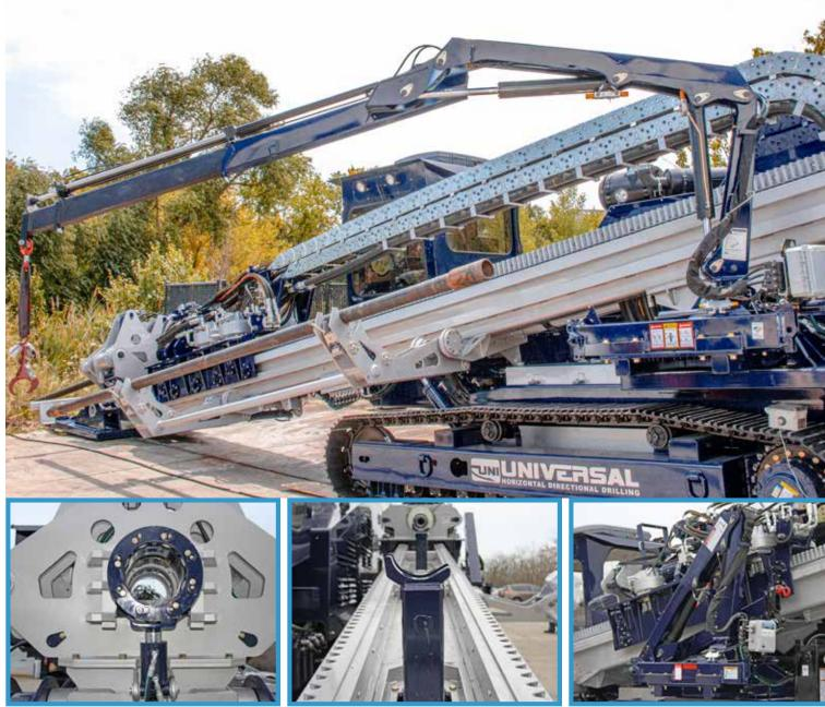
The break-out system features heavy-duty replaceable jaws designed to last and open-top architecture for additional visibility. Also featuring Active Centralizer System (ACS) to reduce wear on drill stems.
