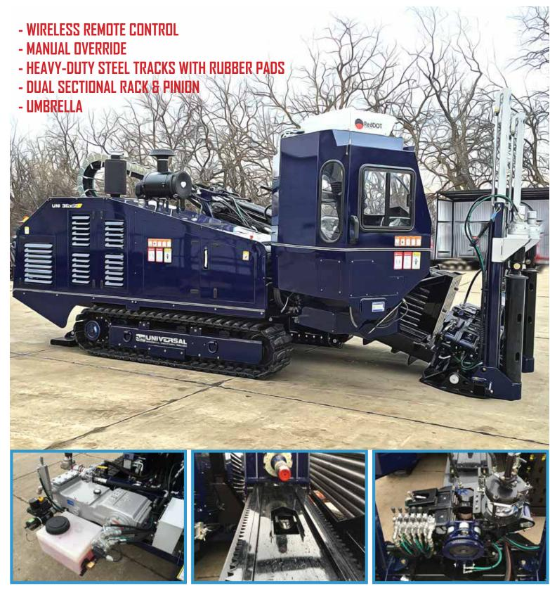
UNI 30x40 come equipped with on-board Kerr mud pump. The build-in mud pump reduces transportation problems and increases maneuverability of the horizontal drilling machine.
