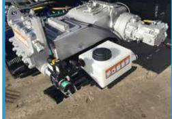
Aplex mud pump, which delivers up to 205 g/min. The build-in mud pump reduces transportation problems and increases maneuverability of the horizontal drilling machine.
