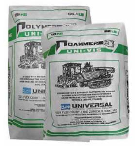
UNI-VIS byopolymer is used for drilling in non-cohesive soil (sand, gravel, etc.) for the purpose of increasing theological characteristics (carrying capacity, gel strength). On high complexity job sites preferably to use it in combination with UNI-PAC; UNI-VIS is a dispersible, non-clarified, high-molecular weight biopolymer used for increasing viscosity in water-base base drilling fluid systems.
