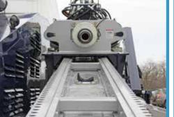
Sectional double rack & pinion can be easily maintained and replaced to reduce downtime and cost of maintenance.
