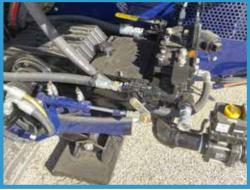
The UNI 25 come equipped with on-board heavy-duty mud pump. This drilling fluid management unit supplies the rig with quality and stable mud during the operational cycle.
