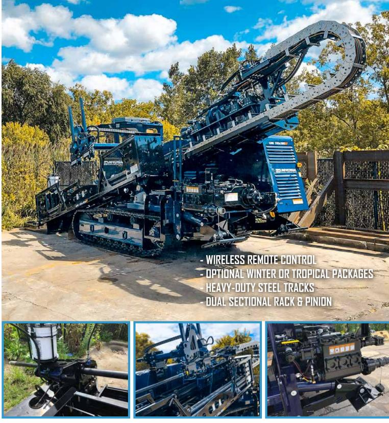
The break-out system features heavy-duty replaceable jaws designed to last and open-top architecture for additional visibility. Also featuring automatic greaser to speed-up working cycle and improve safety.
