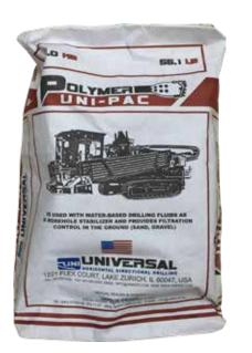
UNI-PAC polyanionic cellulose is effective in low concentrations, with the normal fluid-loss treatment ranging from 0.25 to 1 lb/bbl (0.71 to 2.85 kg/m3). This product is applicable in all water-base muds, ranging from low-solids, non-dispersed polymer systems to high-density, dispersed systems. It is used as a filtrate reducer and borehole stabilizer in water-base drilling applications.
