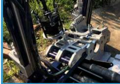
The break-out system features heavy-duty replaceable jaws designed to last and open-top architecture for additional visibility. Also featuring Active Centralizer System (ACS) to reduce wear on drill stems
