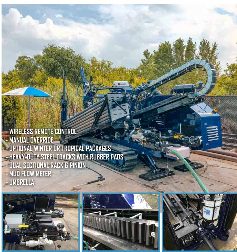
UNI 45x65 come equipped with on-board Kerr mud pump, which delivers up to 115g/min. The build-in mud pump reduces transportation problems and increases maneuverability of the horizontal drilling machine.
